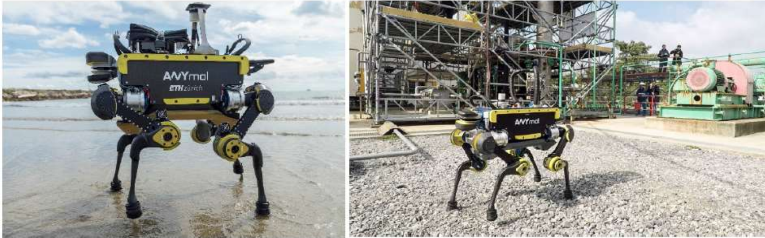
Figure 1. ANYmal is a medium-dog-sized quadrupedal robot. The left images depict the robot in a search and rescue mission in Italy, the right image in an autonomous inspection mission at an industrial site in France.
